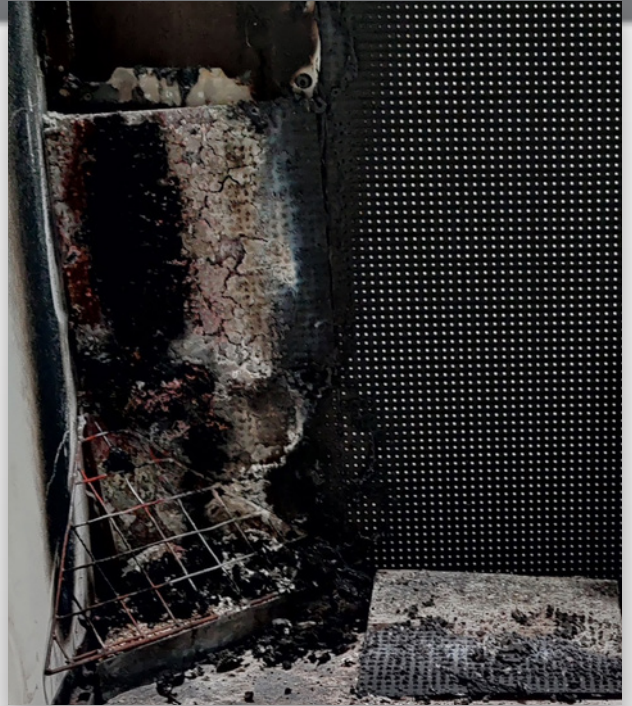
Fig.: Standard LED screen after fire test (SBI)
